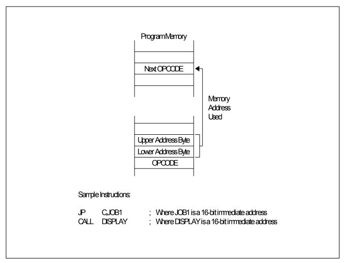
Figure 3-10 Direct Addressing for Load Instructions
