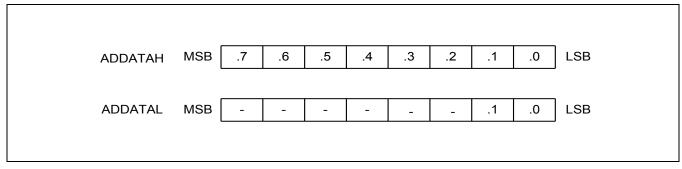
Figure 16-3 A/D Converter Data Register (ADDATAH/L)
