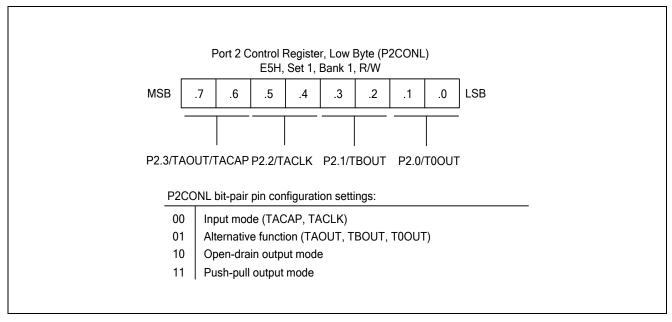
Figure 9-6 Port 2 Low-Byte Control Register (P2CONL)
