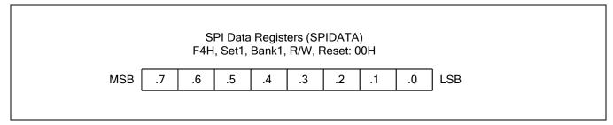
Figure 17-5 SPI Data Register (SPIDATA)
