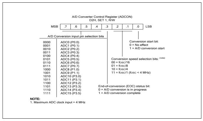
Figure 16-1 A/D Converter Control Register (ADCON)
