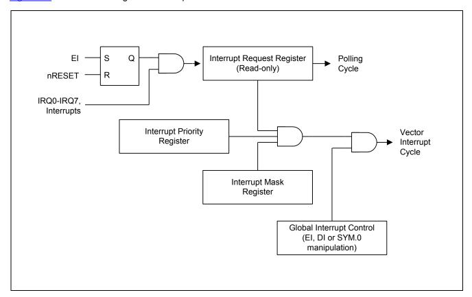
Figure 5-4 Interrupt Function Diagram
