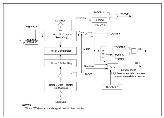
Figure 12-3 Timer 0 Functional Block Diagram
