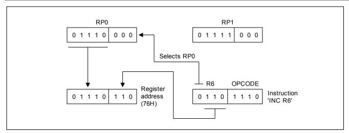
Figure 2-13 4-Bit Working Register Addressing Example
