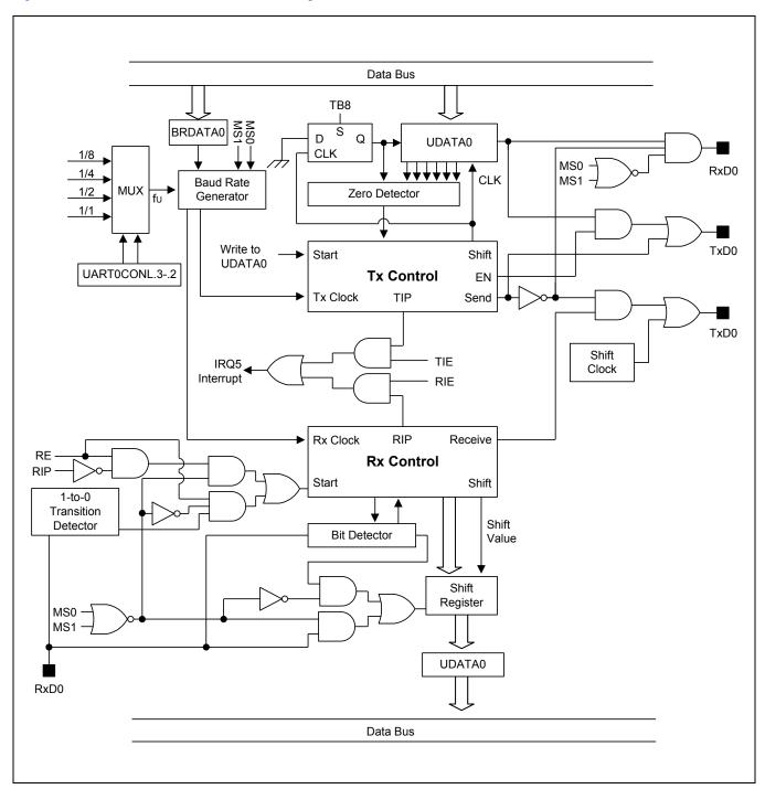
Figure 19-5 UART 0 Functional Block Diagram
