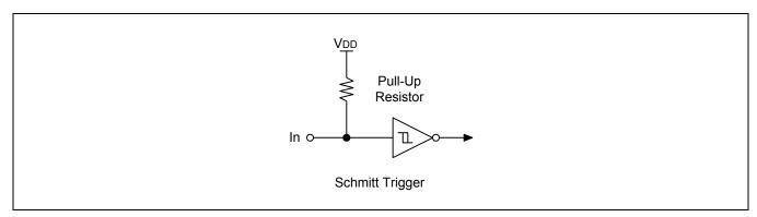
Figure 1-5 Pin Circuit Type B
