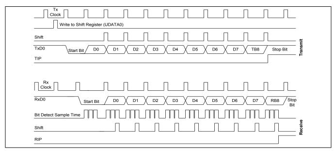
Figure 19-9 Timing Diagram for Serial Port Mode 3 Operation
