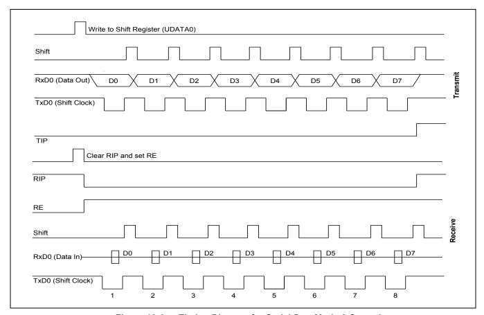
Figure 19-6 Timing Diagram for Serial Port Mode 0 Operation
