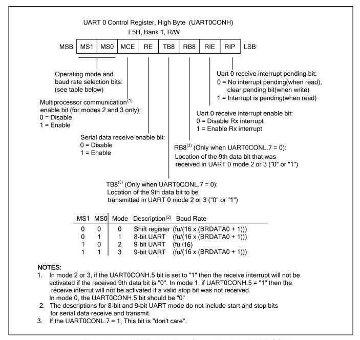
Figure 19-1 UART 0 High Byte Control Register (UART0CONH)
