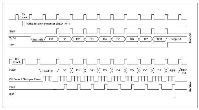
Figure 20-8 Timing Diagram for Serial Port Mode 2 Operation
