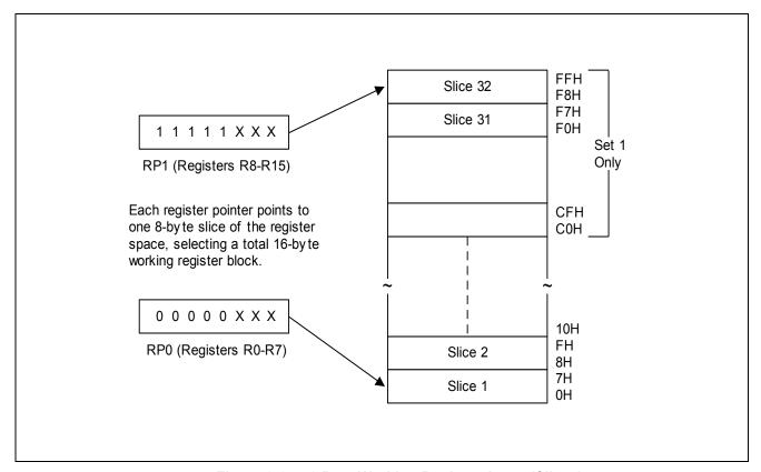
Figure 2-6 8 Byte Working Register Areas (Slices)
