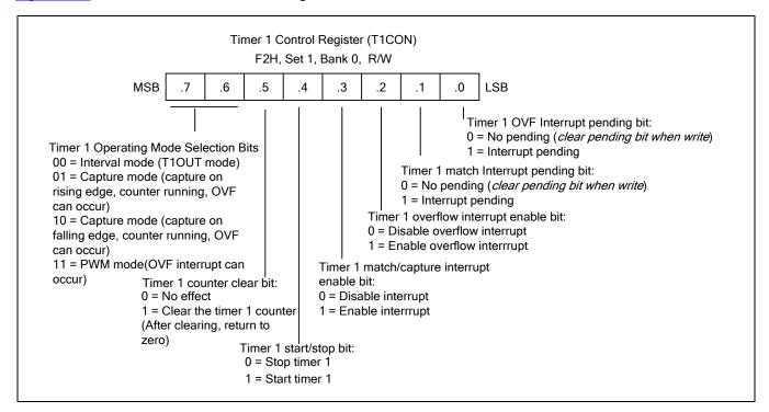
Figure 12-4 Timer 1 Control Register (T1CON)
