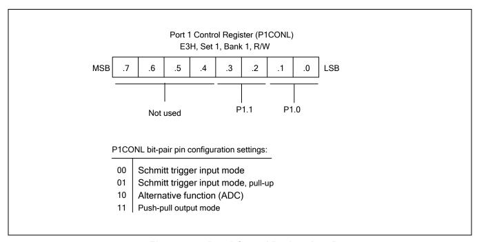
Figure 9-4 Port 1 Control Register Low Byte
