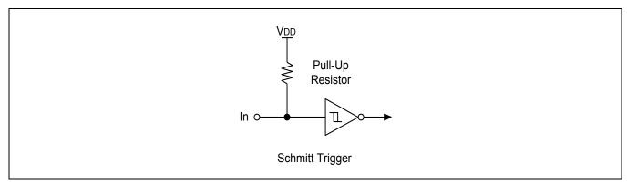
Figure 1-4 Pin Circuit Type A
