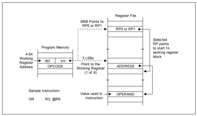
Figure 3-5 Indirect Working Register Addressing to Register File
