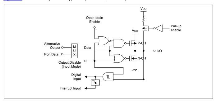
Figure 1-8 Pin Circuit Type D-6 (P2.0-P2.3, P3.6-P3.7)
