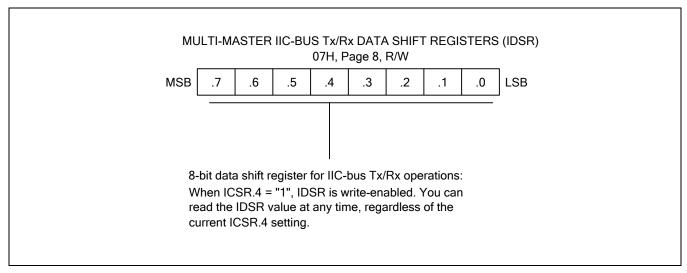
Figure 18-3 Multi-Master IIC-Bus Tx/Rx Data Shift Register (IDSR)
