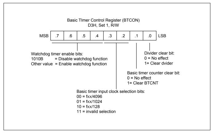
Figure 10-1 Basic Timer Control Register (BTCON)
