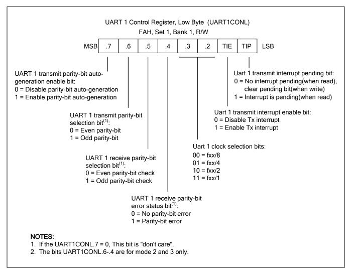
Figure 20-2 UART 1 Low Byte Control Register (UART1CONL)
