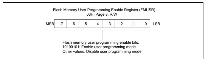
Figure 21-2 Flash Memory User Programming Enable Register (FMUSR)
