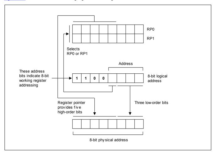
Figure 2-14 8-Bit Working Register Addressing
