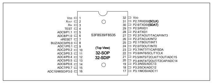
Figure 25-1 S3F8S39/S3F8S35 Pin Assignments (32-SOP/32-SDIP)
