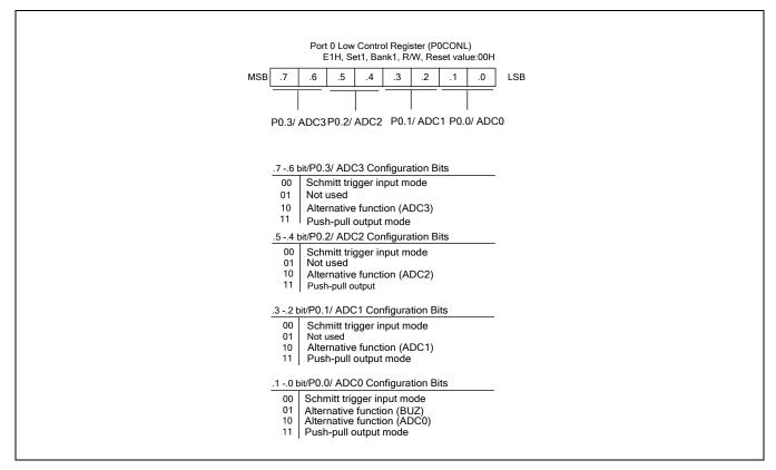
Figure 9-2 Port 0 Control Register Low Byte (P0CONL)
