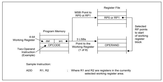
Figure 3-2 Working Register Addressing
