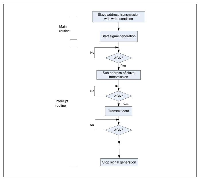
Figure 18-11 Write Operation Sequence
