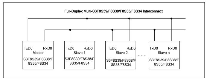
Figure 19-10 Connection Example for Multiprocessor Serial Data Communications
