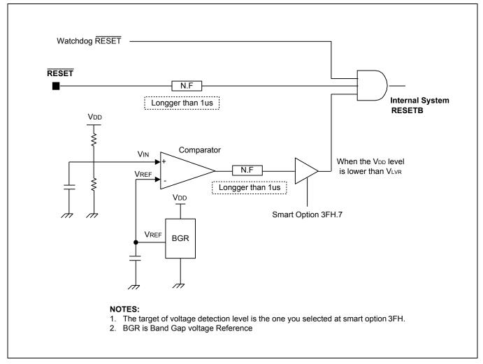
Figure 8-1 Low Voltage Reset Circuit
