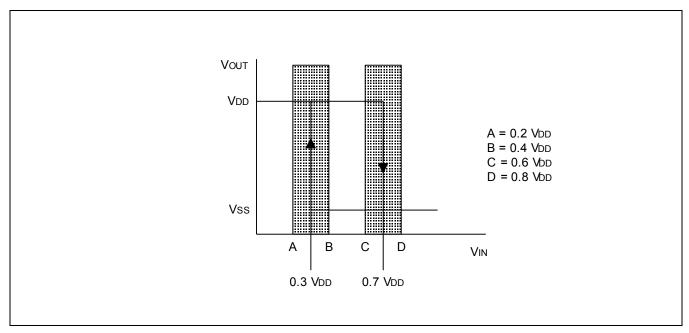
Figure 23-3 Schmitt Trigger Input Characteristics Diagram
