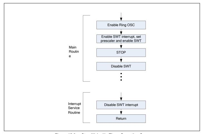
Figure 15-3 Stop Wake-Up Timer Operation Sequence
