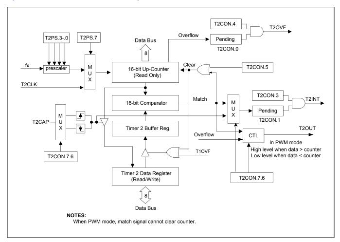
Figure 12-9 Timer 2 Functional Block Diagram
