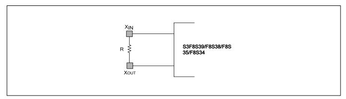
Figure 7-1 Main Oscillator Circuit (RC Oscillator with Internal Capacitor)
