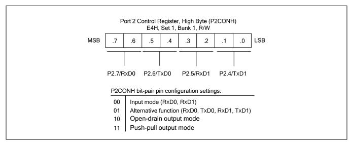
Figure 9-5 Port 2 High-Byte Control Register (P2CONH)
