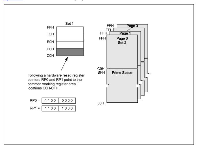
Figure 2-11 Common Working Register Area
