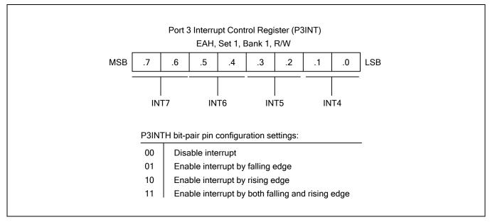
Figure 9-11 Port 3 Interrupt Control Register (P3INT)
