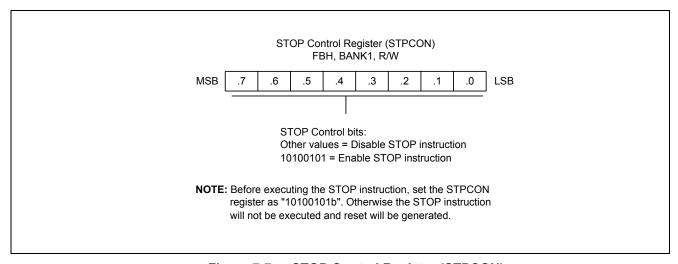
Figure 7-7 STOP Control Register (STPCON)
