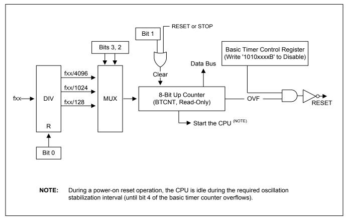
Figure 10-2 Basic Timer Block Diagram
