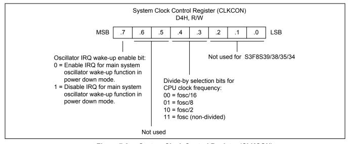
Figure 7-3 System Clock Control Register (CLKCON)
