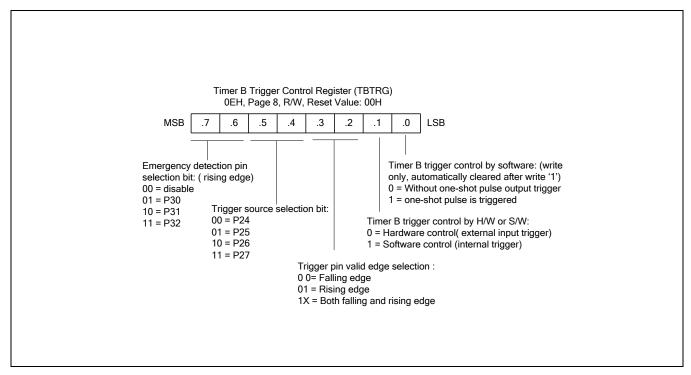
Figure 13-2 Timer B Trigger Register (TBTRG)
