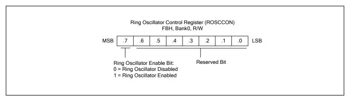
Figure 7-6 Ring Oscillator Control Register (ROSCCON)
