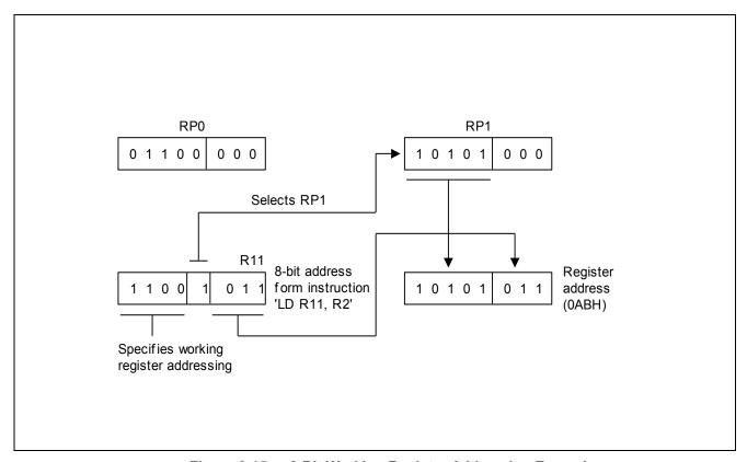
Figure 2-15 8-Bit Working Register Addressing Example
