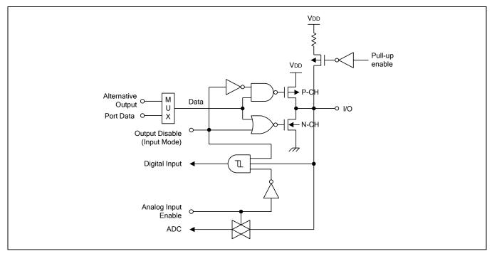
Figure 1-10 Pin Circuit Type E-1 (P0, P1)
