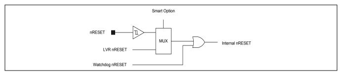
Figure 8-2 Reset Block Diagram
