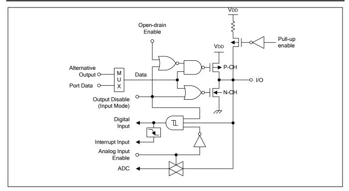
Figure 1-7 Pin Circuit Type D-5 (P3.4-P3.5)
