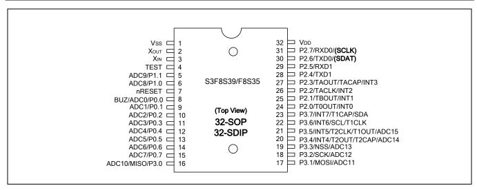
Figure 1-2 S3F8S39/S3F8S35 Pin Assignment (32-SOP/SDIP)
