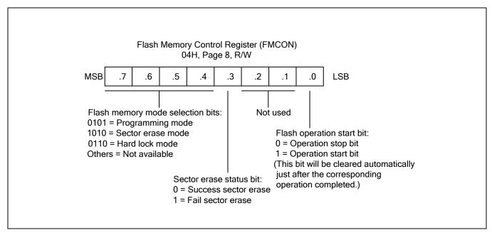
Figure 21-1 Flash Memory Control Register (FMCON)
