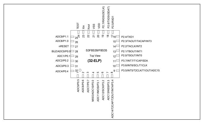
Figure 1-3 S3F8S39/S3F8S35 Pin Assignment (32-ELP)
