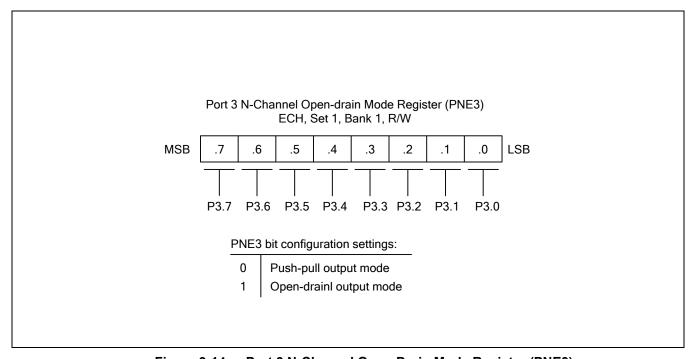
Figure 9-14 Port 3 N-Channel Open-Drain Mode Register (PNE3)
