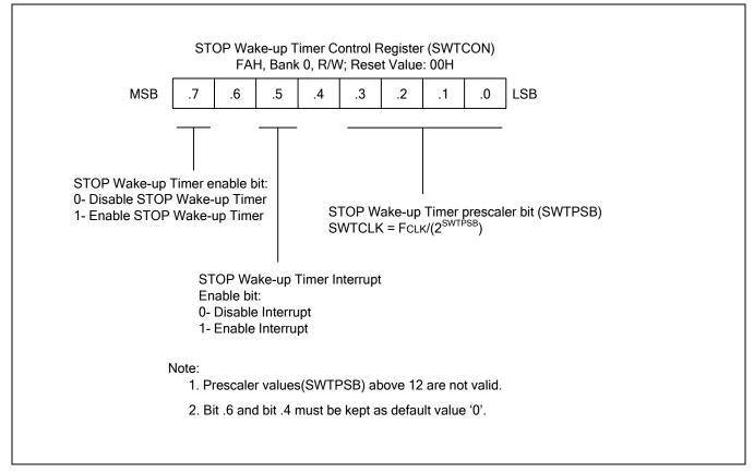
Figure 15-1 Stop Wake-Up Timer Control Register (SWTCON)
