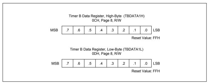
Figure 13-4 Timer B Data Registers (TBDATA1H/L)
