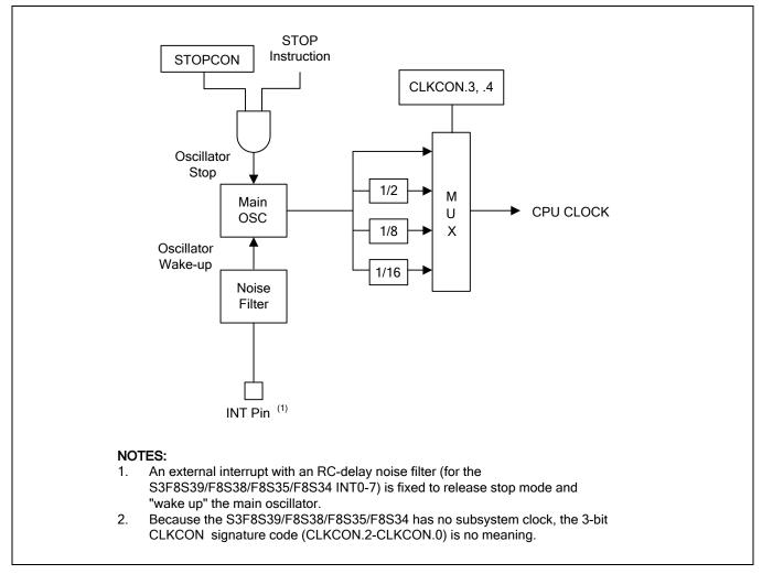
Figure 7-8 System Clock Circuit Diagram
