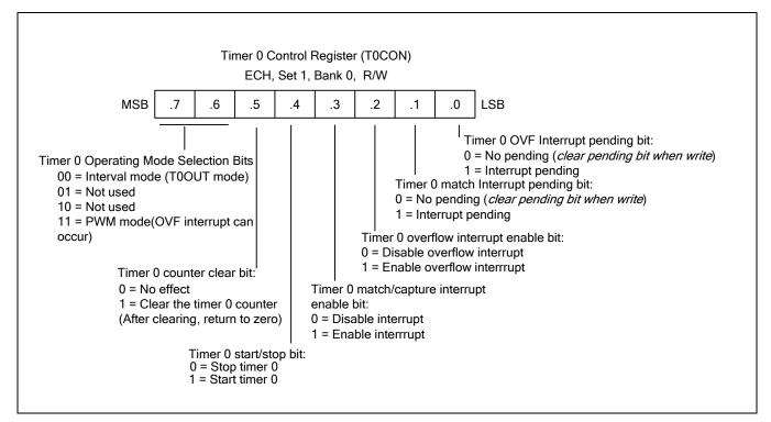
Figure 12-1 Timer 0 Control Register (T0CON)
