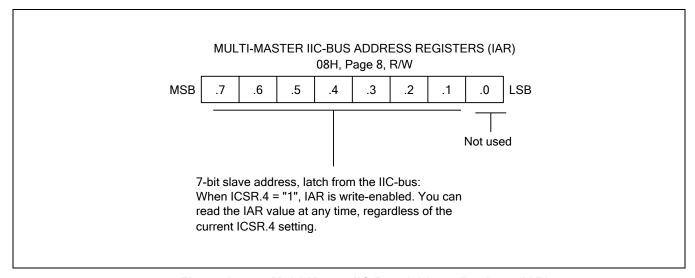
Figure 18-4 Multi-Master IIC-Bus Address Register (IAR)
