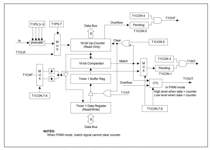
Figure 12-6 Timer 1 Functional Block Diagram
