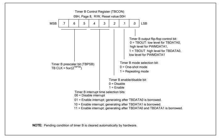
Figure 13-1 Timer B Control Register
