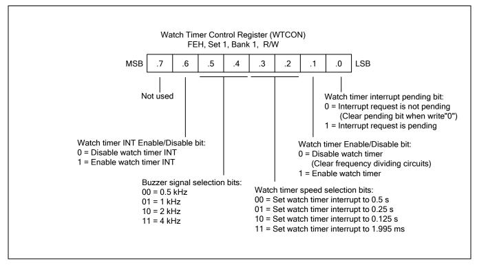
Figure 14-1 Watch Timer Control Register (WTCON)
