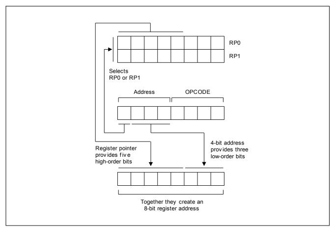
Figure 2-12 4-Bit Working Register Addressing
