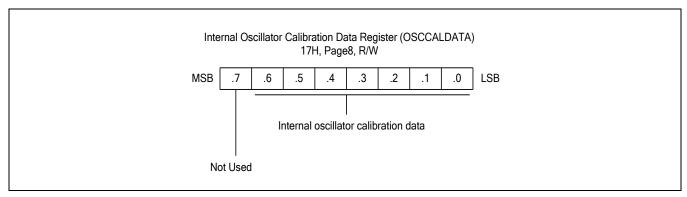
Figure 7-5 Internal Oscillator Calibration Data Register (OSCCALDATA)
