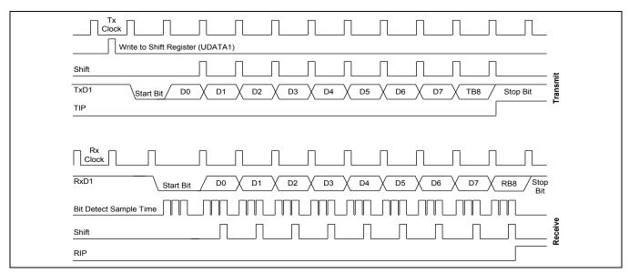
Figure 20-9 Timing Diagram for Serial Port Mode 3 Operation
