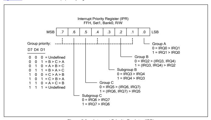
Figure 5-8 Interrupt Priority Register (IPR)
