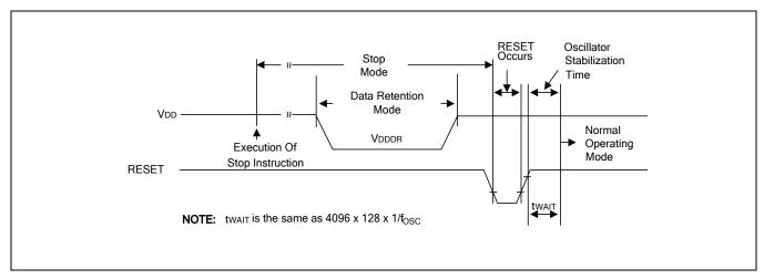
Figure 23-4 Stop Mode Release Timing When Initiated by a RESET
