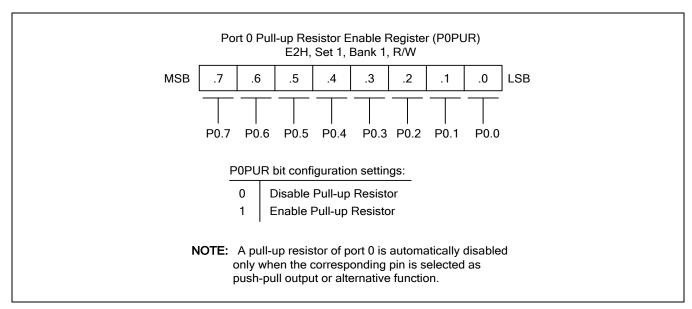
Figure 9-3 Pull-up Resistor Enable Register (P0PUR)
