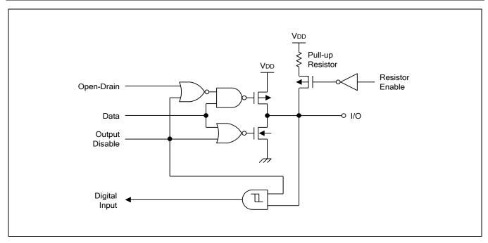
Figure 1-11 Pin Circuit Type E-2 (P2.4-P2.7)
