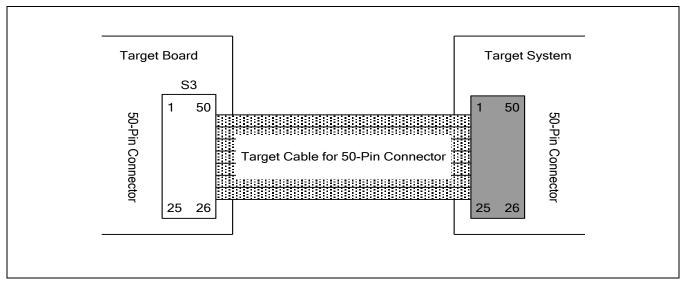
Figure 26-5 S3F8S39/S3F8S35 Probe Adapter for 50 Pin Package
