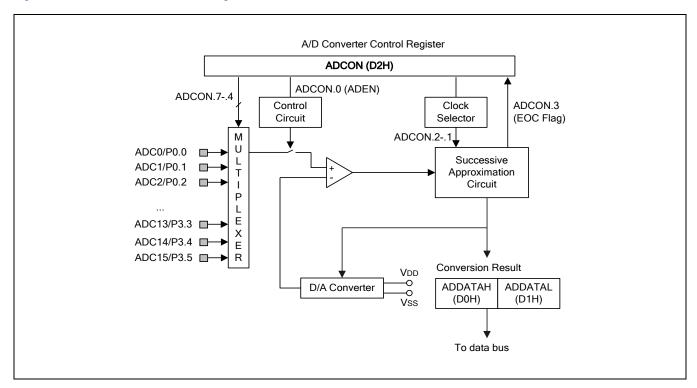
Figure 16-2 A/D Converter Circuit Diagram
