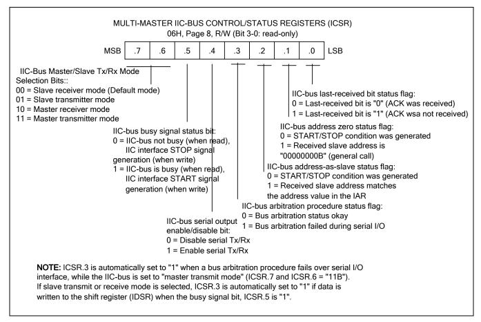
Figure 18-2 Multi-Master IIC-Bus Control/Status Register (ICSR)
