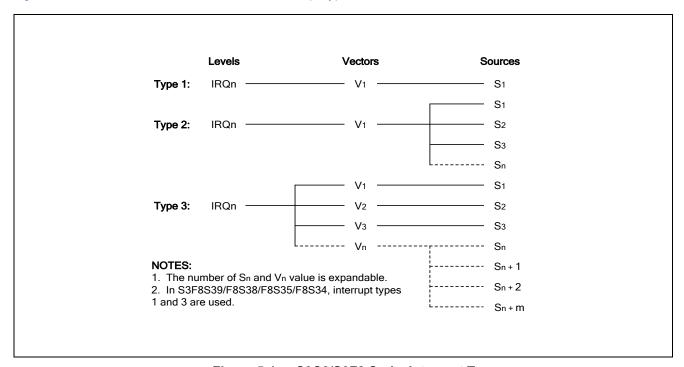
Figure 5-1 S3C8/S3F8 SeriesInterrupt Types
