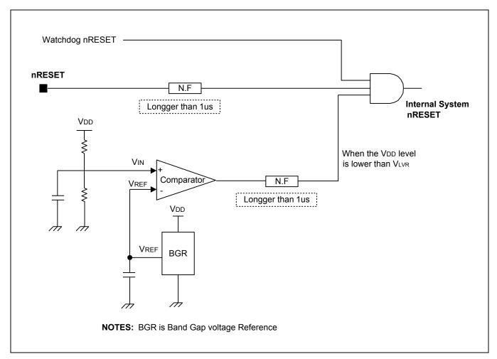
Figure 22-1 Low Voltage Reset Circuit
