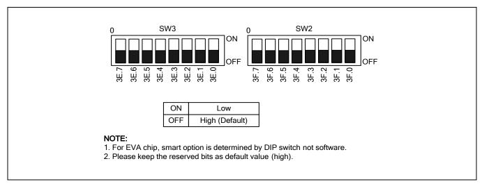
Figure 26-3 DIP Switch for Smart Option
