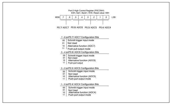
Figure 9-1 Port 0 Control Register High Byte (P0CONH)
