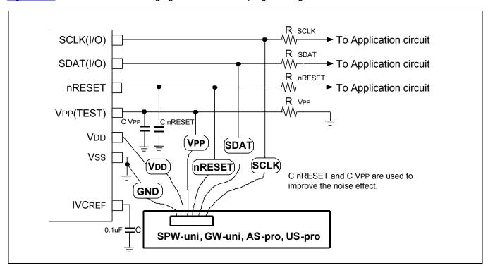
Figure 25-4 PCB Design Guide for On-Board Programming
