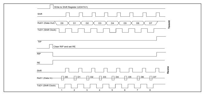
Figure 20-6 Timing Diagram for Serial Port Mode 0 Operation
