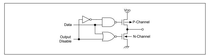
Figure 1-6 Pin Circuit Type C
