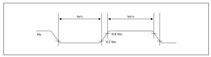
Figure 23-1 Input Timing Measurement Points
