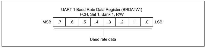
Figure 20-4 UART 1 Baud Rate Data Register (BRDATA1)
