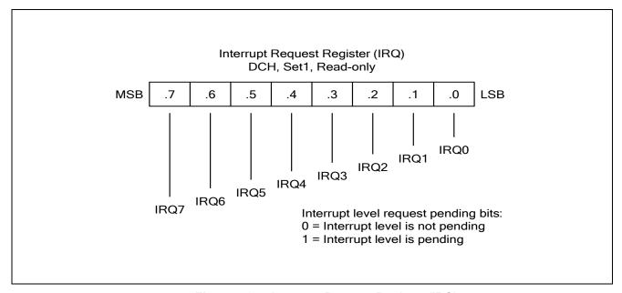
Figure 5-9 Interrupt Request Register (IRQ)
