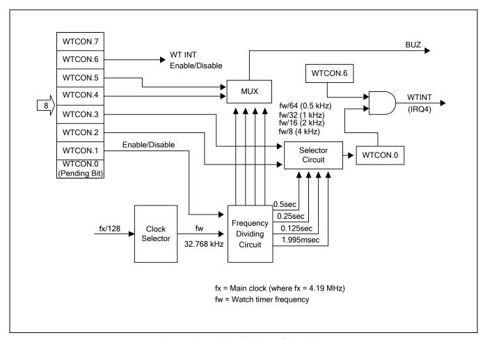
Figure 14-2 Watch Timer Circuit Diagram
