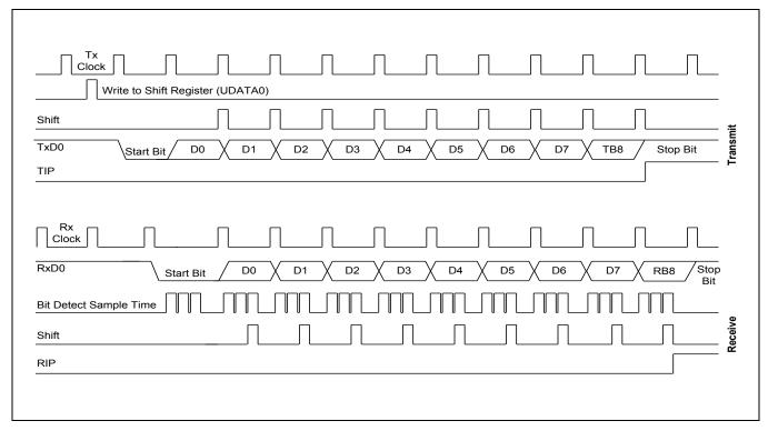
Figure 19-8 Timing Diagram for Serial Port Mode 2 Operation
