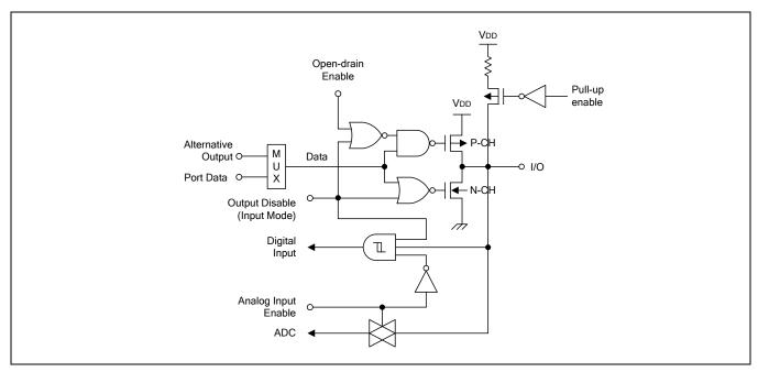
Figure 1-9 Pin Circuit Type E (P3.0-P3.3)
