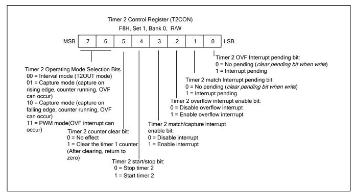
Figure 12-7 Timer 2 Control Register (T2CON)
