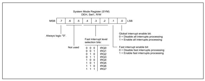
Figure 5-5 System Mode Register (SYM)
