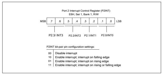
Figure 9-7 Port 2 Interrupt Control Register (P2INT)
