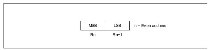
Figure 2-9 16-Bit Register Pair
