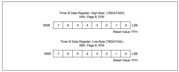
Figure 13-3 Timer B Data Registers (TBDATA0H/L)
