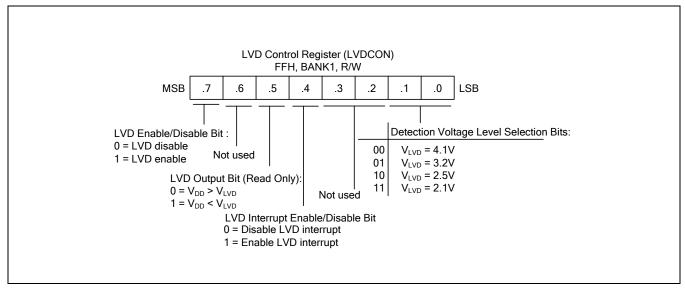
Figure 22-3 Low Voltage Detect Control Register (LVDCON)
