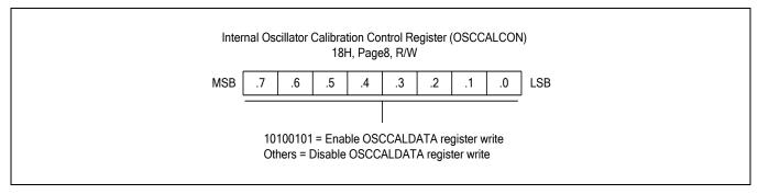
Figure 7-4 Internal Oscillator Calibration Control Register (OSCCALCON)
