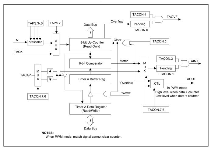
Figure 11-3 Timer A Functional Block Diagram
