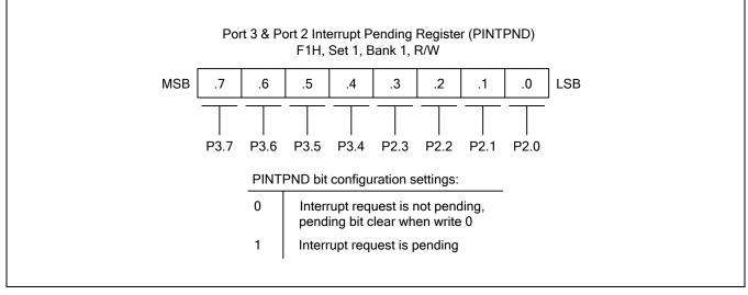
Figure 9-12 Port 3 & Port 0 Interrupt Pending Register (PINTPND)
