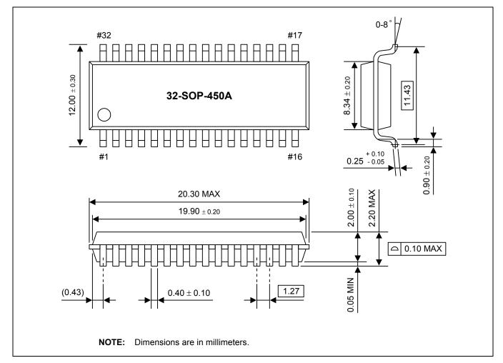
Figure 24-1 32-SOP-450A Package Dimensions
