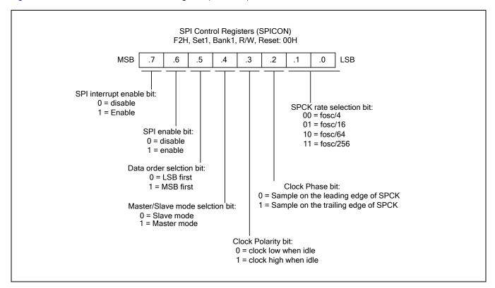
Figure 17-3 SPI Control Register (SPICON)
