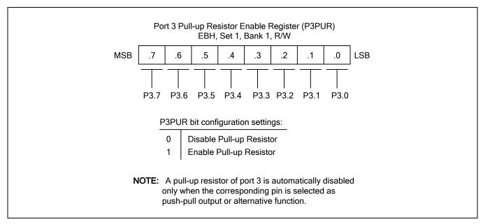
Figure 9-13 Port 3 Pull-Up Resistor Enable Register (P3PUR)
