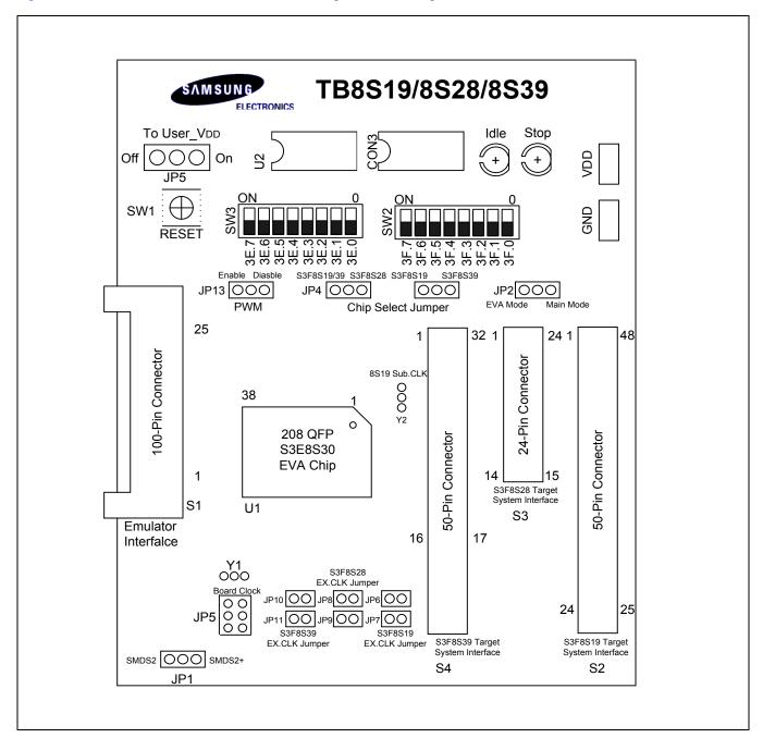
Figure 26-2 TB8S19/8S28/8S39 Target Board Configuration
