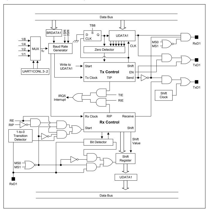
Figure 20-5 UART 1 Functional Block Diagram
