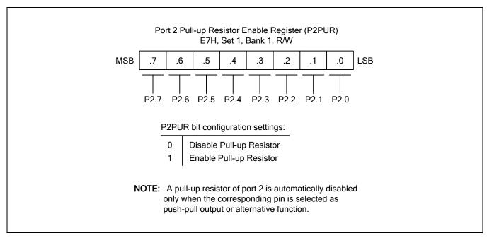
Figure 9-8 Port 2 Pull-Up Resistor Enable Register (P2PUR)
