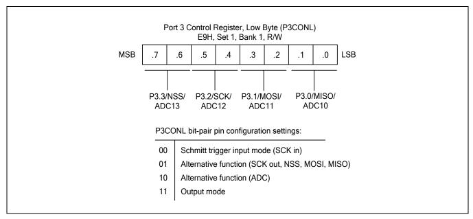
Figure 9-10 Port 3 Low-Byte Control Register (P3CONL)
