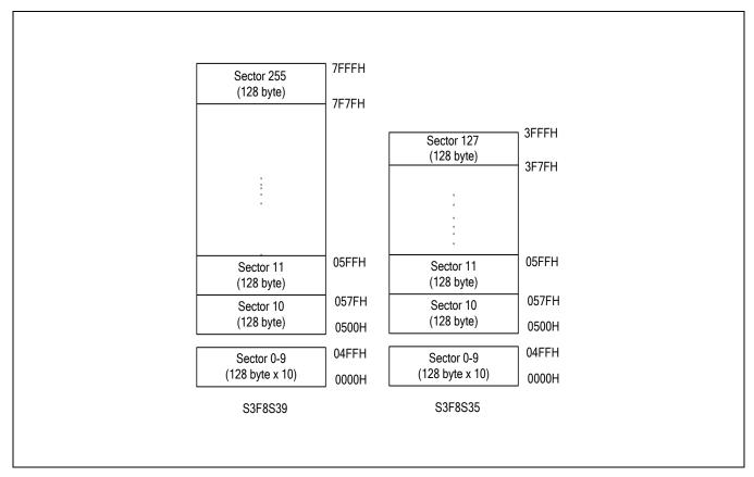
Figure 21-6 Sector Configurations in User Program Mode
