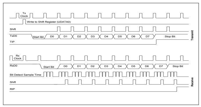
Figure 19-7 Timing Diagram for Serial Port Mode 1 Operation
