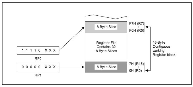
Figure 2-8 Non-Contiguous 16 Byte Working Register Block
