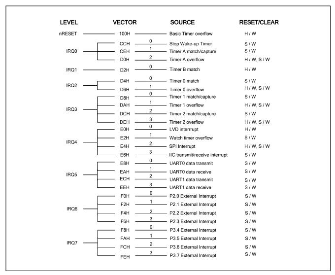
Figure 5-2 S3F8S39/S3F8S35 Interrupt Structure
