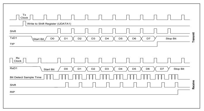
Figure 20-7 Timing Diagram for Serial Port Mode 1 Operation
