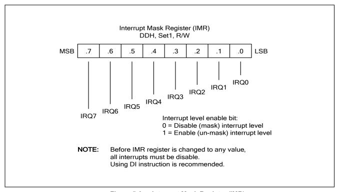
Figure 5-6 Interrupt Mask Register (IMR)
