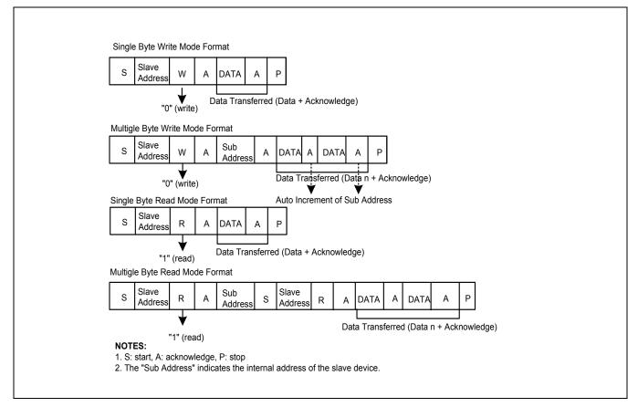
Figure 18-9 IIC-Bus Interface Data Formats
