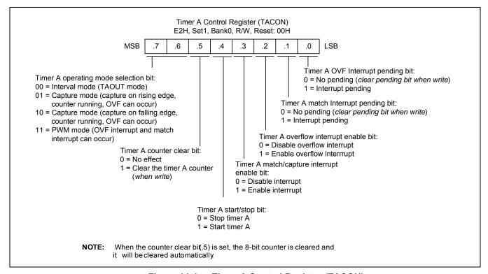
Figure 11-1 Timer A Control Register (TACON)
