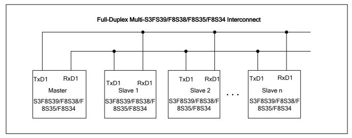
Figure 20-10 Connection Example for Multiprocessor Serial Data Communications
