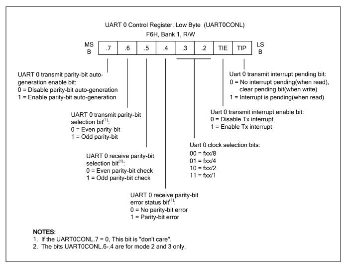
Figure 19-2 UART 0 Low Byte Control Register (UART0CONL)
