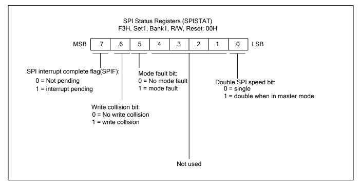
Figure 17-4 SPI Status Register (SPISTAT)
