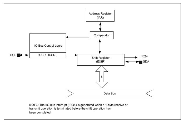
Figure 18-5 IIC-Bus Block Diagram
