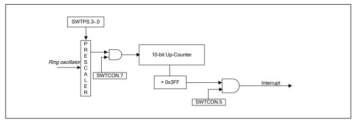
Figure 15-2 Stop Wake-Up Timer Functional Block Diagram
