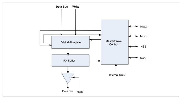
Figure 17-1 SPI Block Diagram
