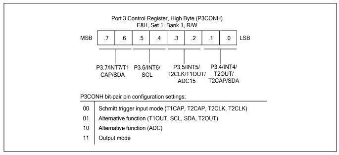
Figure 9-9 Port 3 High-Byte Control Register (P3CONH)
