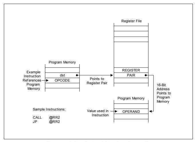
Figure 3-4 Indirect Register Addressing to Program Memory
