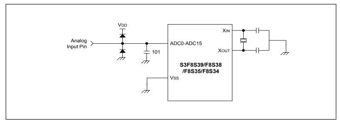
Figure 16-5 Recommended A/D Converter Circuit for Highest Absolute Accuracy
