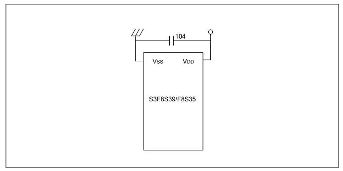
Figure 23-7 The Circuit Diagram to Improve EFT Characteristics
