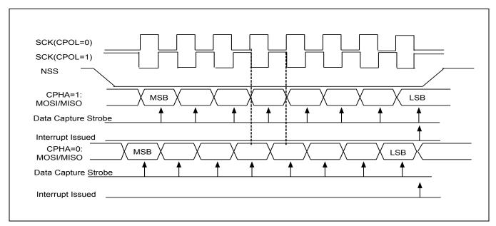
Figure 17-2 SPI Data Timing
