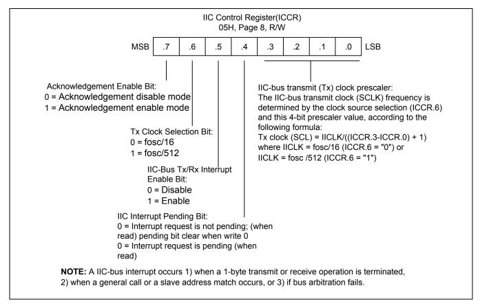
Figure 18-1 Multi-Master IIC-Bus Control Register (ICCR)
