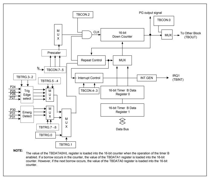
Figure 13-5 Timer B Functional Block Diagram
