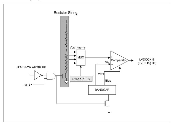
Figure 22-2 Low Voltage Detect (LVD) Block Diagram
