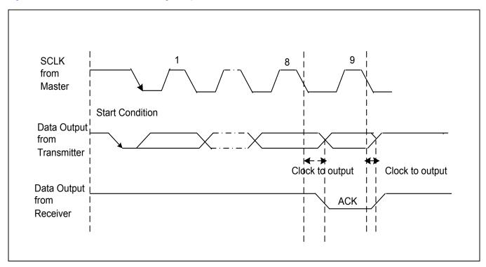
Figure 18-10 Acknowledge Response from Receiver
