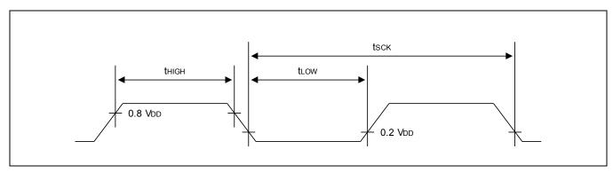
Figure 23-5 Waveform for UART Timing Characteristics
