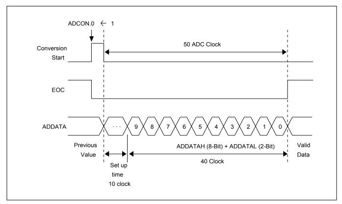
Figure 16-4 A/D Converter Timing Diagram
