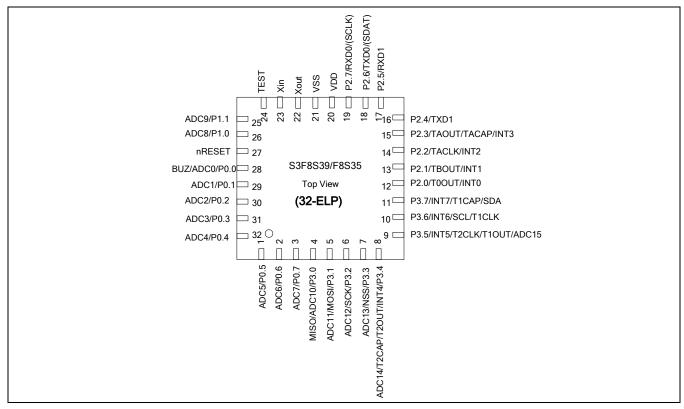
Figure 25-2 S3F8S39/S3F8S35 Pin Assignments (32-ELP)
