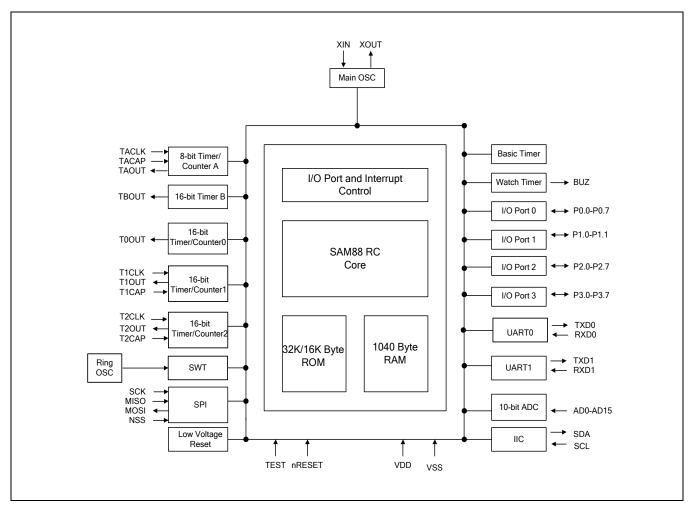
Figure 1-1 S3F8S39/S3F8S35 Block Diagram
