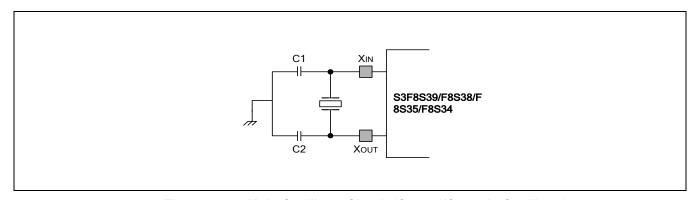
Figure 7-2 Main Oscillator Circuit (Crystal/Ceramic Oscillator)
