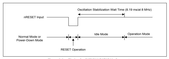
Figure 8-3 Timing for S3F8S39/S3F8S35 after reset
