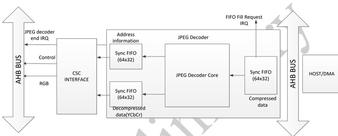
Figure 22-1 JPEG Decoder Block Diagram
