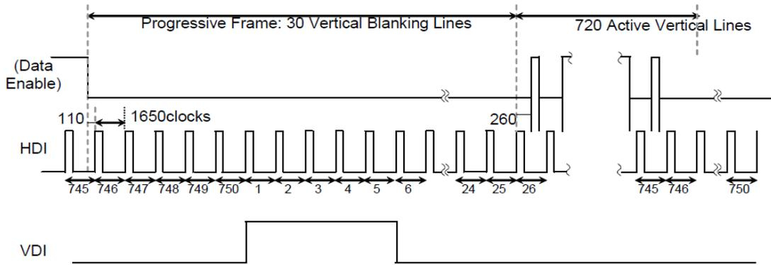
Figure 19-4 Input Video data Vsync Timing
