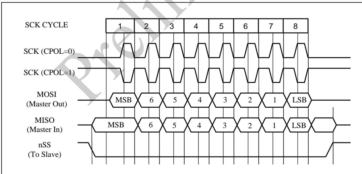
Figure 30-3 Transfer Timing when CPHA = '0'
