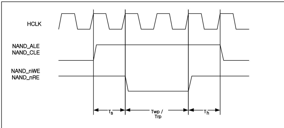
Figure 11-2 Read/Write Timing Diagram of NAND Flash Memory
