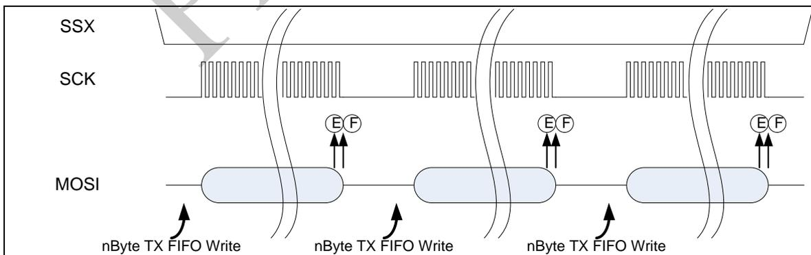
Figure 30-6 n-Bytes Transfer vs. Status and Interrupt
