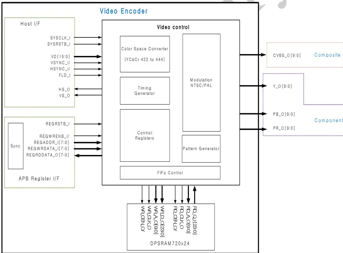
Figure 18-1 Video Encoder Block Diagram
