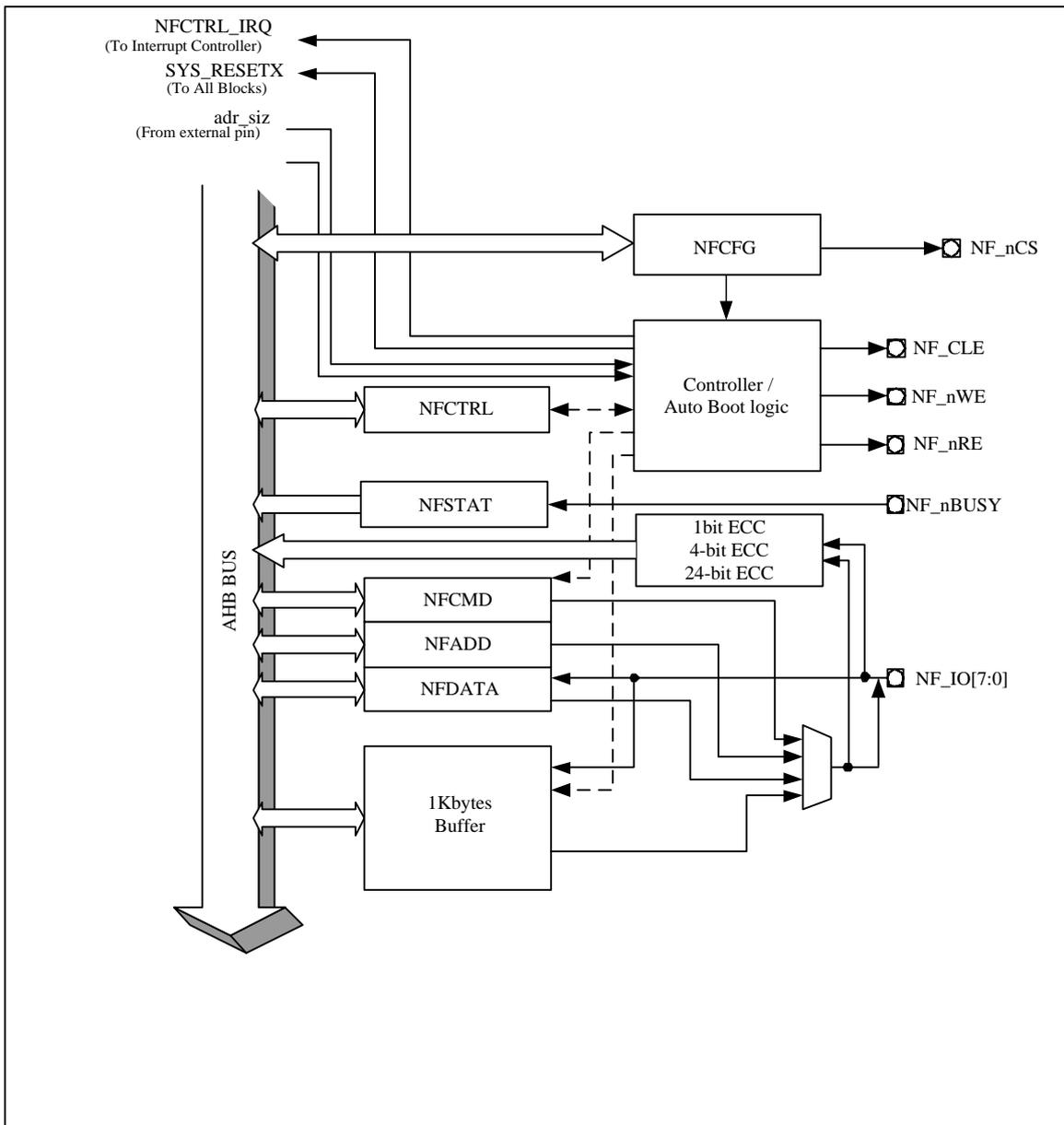
Figure 11-1 NAND Flash Controller Block Diagram
