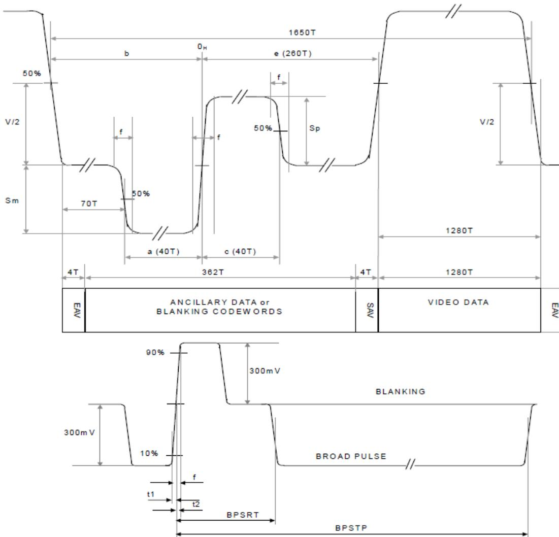
Figure 19-6 Output Video Data HSync Timing (60Mhz)
