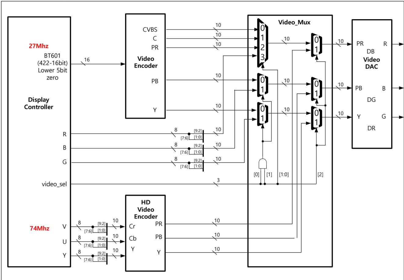
Figure 17-2 Block diagram of the Video Selector
