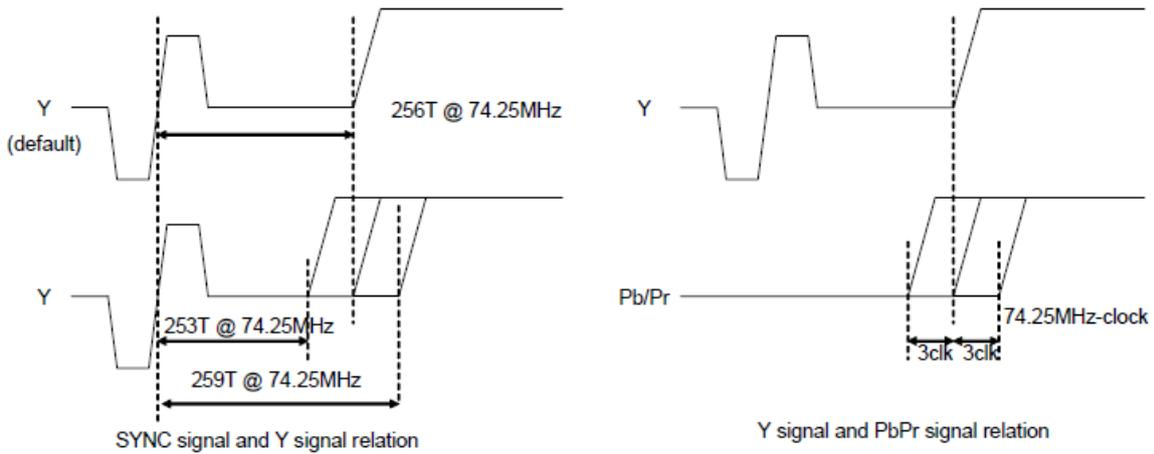
Figure 19-8 Output Video Data HSync table (60Mhz)
