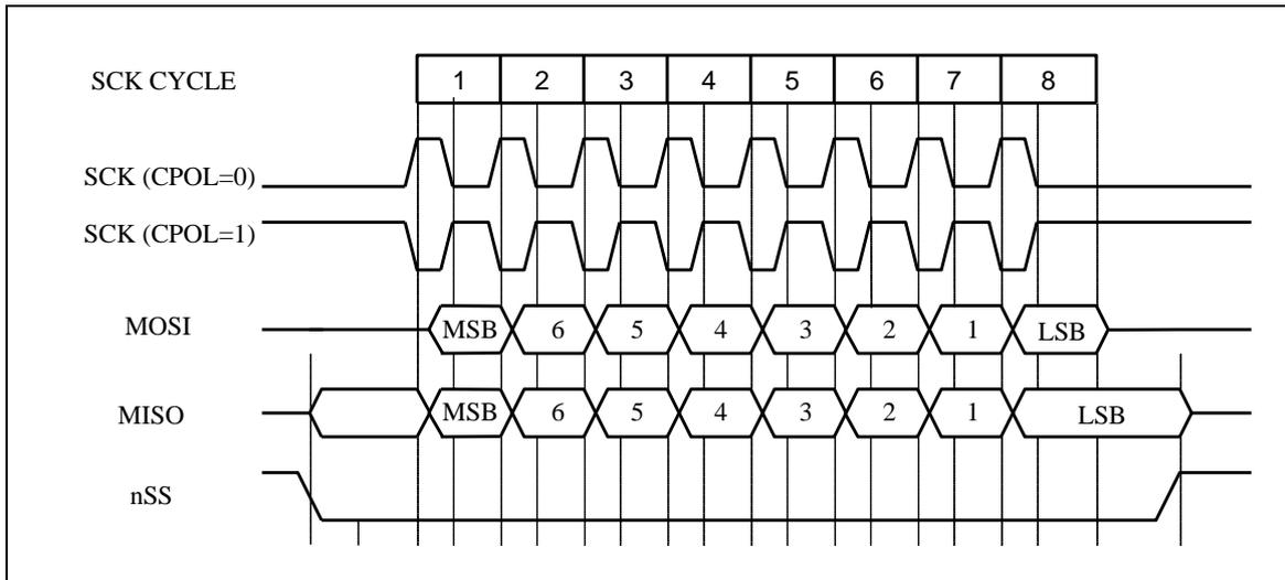
Figure 30-4 Transfer Timing when CPHA = '1'
